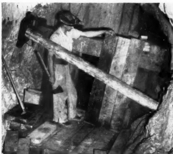
STOPE PREPARATION is done by two men who lace off chutes, and seal area with burlap to prevent water and sand seepage. Stulls are for temporary support of hanging wall.
